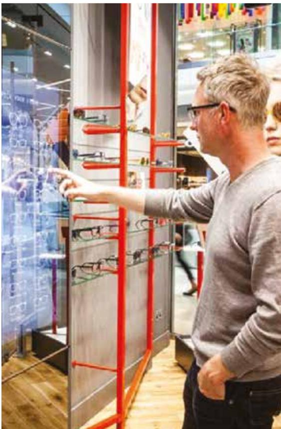
A Zytronic touch sensor sits behind a mirror-finished toughened glass frontage, combined with a forward facing HD camera
